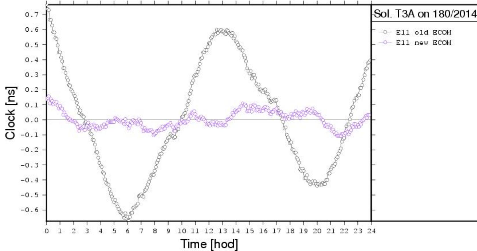
DOY 14/180: Beta-angle is low (i.e., cross-section of satellite body wrt. the Sun varies periodically during each orbital revolution)
