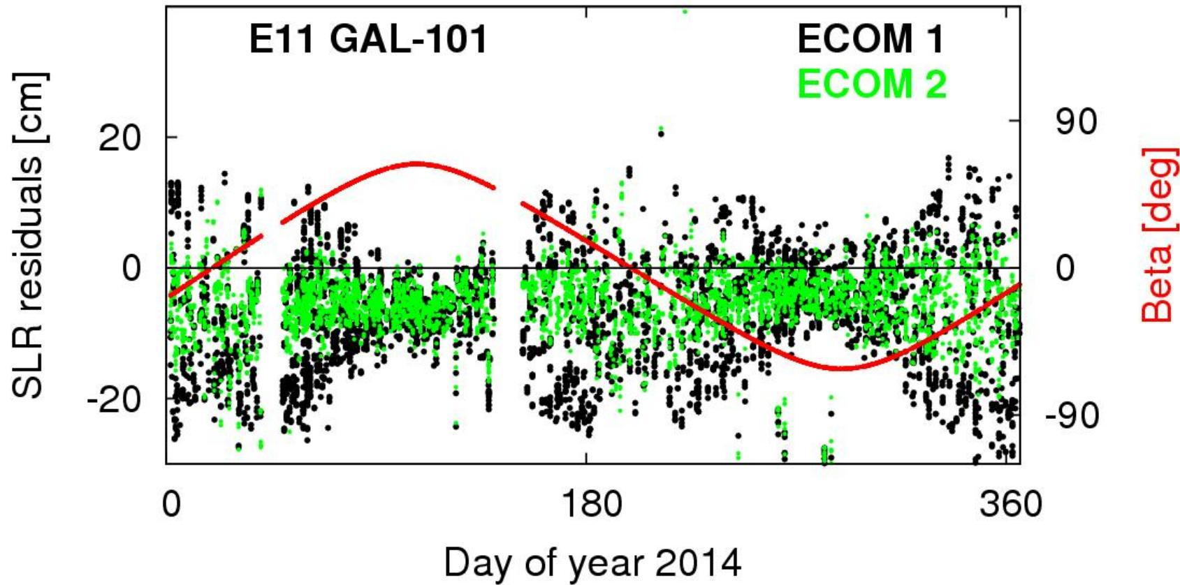
=> Significant reduction of size and dependency of SLR residuals on the Beta-angle (elevation of the Sun above the orbital plane)
