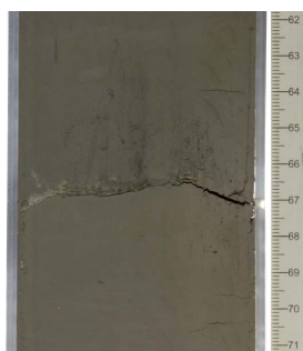
Figure F8. Erosion surface between 2 clay units, Hole U1433A, Unit I (16H-6A, 62–71 cm). Note the thin silt developed on the left side of the core along the contact.
