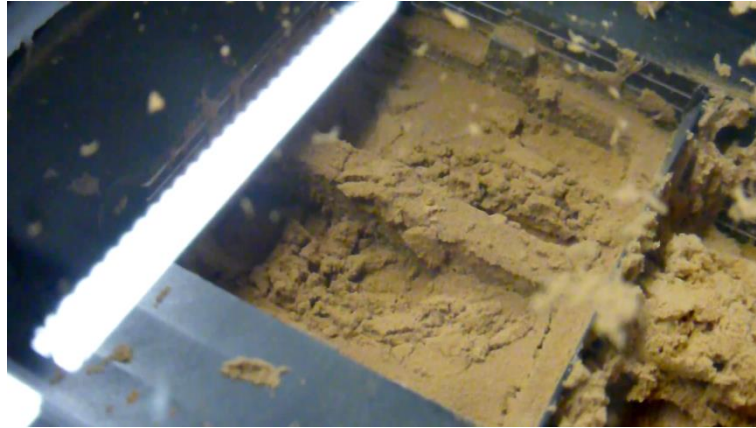
Video 10 : Slow motion capture (200 fps) of an ejection event occurring on the sublimation residue of a sample of water ice inter-mixed with tholins, olivine and smectite seen on Video 7 (tholins-minerals-inter-mixture-1 sample, cf. Table 1). The speed of the ejected particles has been estimated to be around 1.0 \pm 0.1 \text{ m s}^{-1} . The video was recorded with a rate of 200 frames per second. So the time separating each frame of this video is 5 ms. The sample holder is 6 cm wide.
