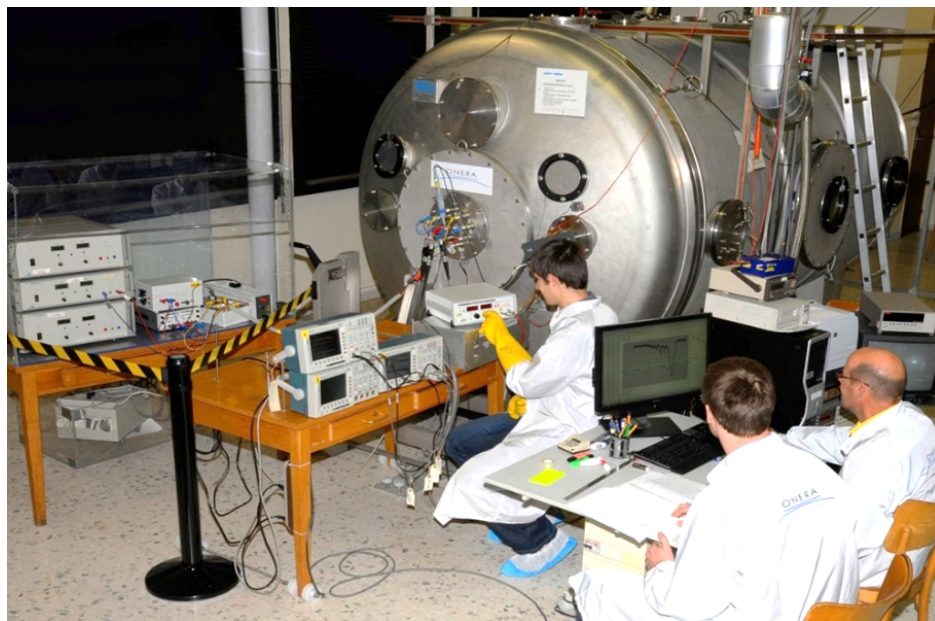
Figure 4.10: Photograph of the ONERA/JONAS facility used for the COPS plasma test. From Inguibert and Murat (2015).
