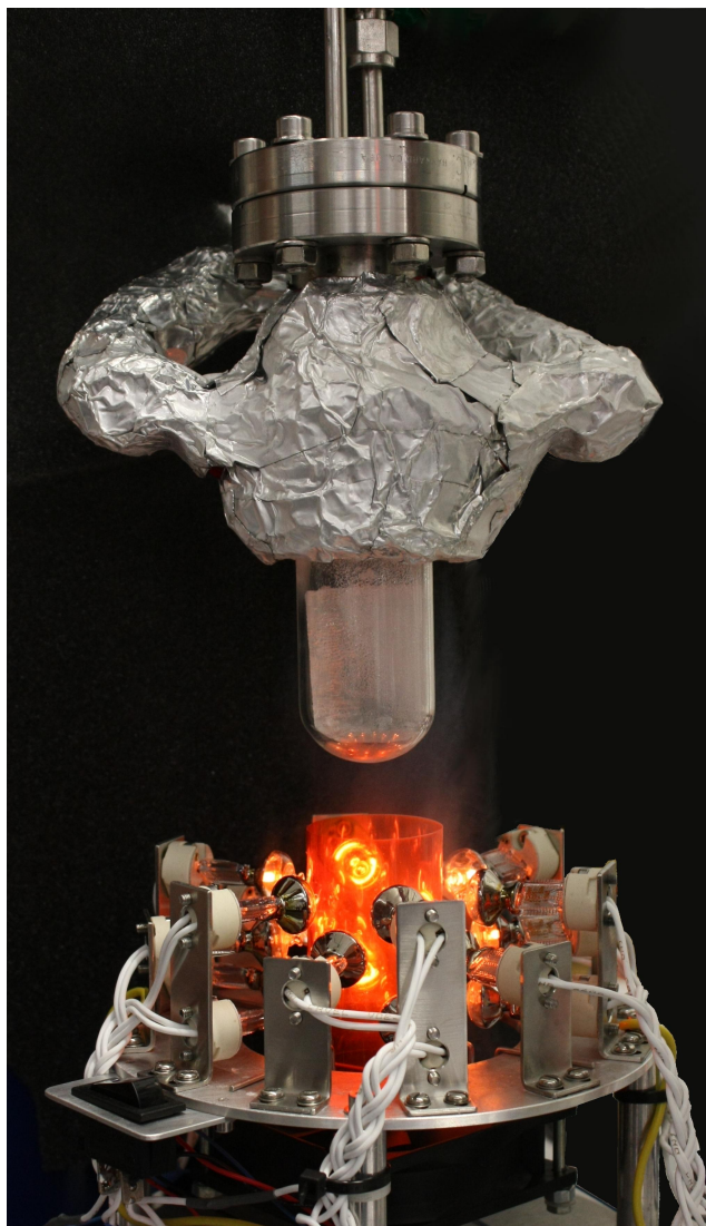
Fig. 2. Photo showing the sublimation vessel with a loaded ice sample and the infrared source. The cooling jacket starts just above the ice sample and a cold air stream is fed in from both sides. The infrared source consists of 18 bulbs mounted on a holder, and the red UV filter visible in the central part. For the sublimation of the ice sample the infrared source is moved upwards, hence the section with sample is surrounded by the bulbs.
