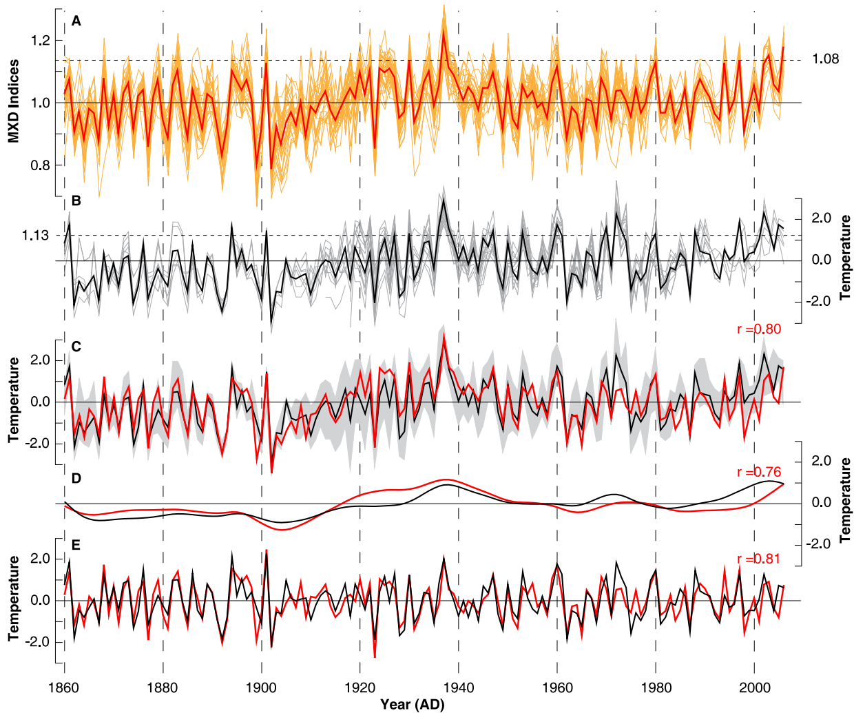
Figure 2. Agreement between high to low frequency variability of the tree-ring proxy and instrumental target data over the past 150 years. (A) Site and subsets RCS chronologies (orange) and their mean (red). (B) JJA temperatures of eight instrumental stations (grey), and the grid-box mean (black). Dashed horizontal lines and corresponding values indicate the mean of the last decade (1997–2006). (C) Instrumental gridded (black) and reconstructed proxy (red) temperatures superimposed on the min/max range of the station measurements (grey shading), expressed as anomalies from 1961–1990, and split into (D) 20-year low-pass and (E) 20-year high-pass components. Correlation (1860–2006) of the unfiltered and filtered timeseries is shown in red. doi:10.1371/journal.pone.0025133.g002
