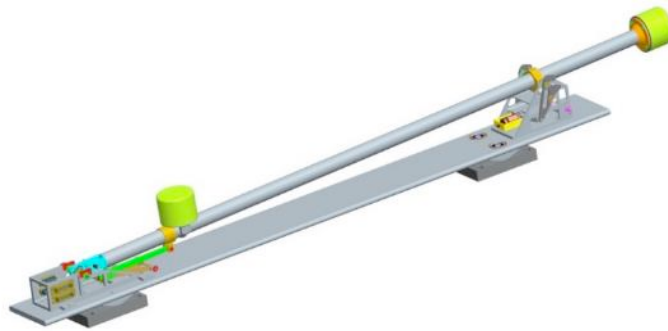
Figure 8: Example of developed and tested boom with two flux-gate magnetometers for the KOMPSAT mission.
