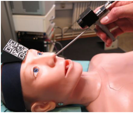
Fig. 1 Laboratory setup of the single camera, marker based surgical navigation system
