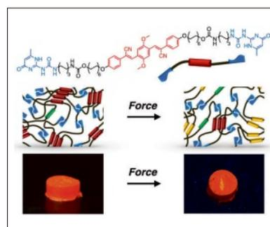
The new material exhibits the characteristic thermo-mechanical properties of a supramolecular polymer, offers three different emission colors in the solid state and exhibits both mechano- and thermo-responsive luminescence.
