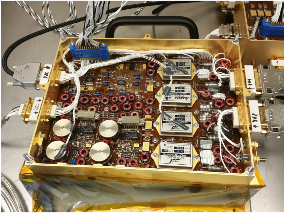
Fig. 18 The Power Converter Module after integration into its frame
