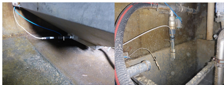
Fig. 3 Technical device to measure pH-value in the liquid feed. A pH-value probe (1) permanently measures the pH-value of the feed soup in the mixing vat. An automatic addition of acid from a dosing feeder (2) ensures a constant pH-value in the liquid feed
