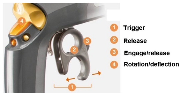
Fig. 2 Kymerax handle: 1 Trigger for opening and closing instrument. 2 Release of engaged trigger. 3 Engage/release trigger. 4 Buttons for tip rotation and deflection. (kymerax.info)
