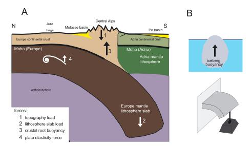
**Figure 4.** (a) Main forces in dynamic equilibrium driving the central Alpine orogeny since collision times. (b) The main driving forces for mountain building and for subduction are the buoyancy of the crust and the slab pull by the mantle lithosphere, respectively, the latter of which has a higher density than the underlying asthenosphere. Depending on its elasticity, the plate reacts to the bending moment by bulging (Royden, 1993b).
