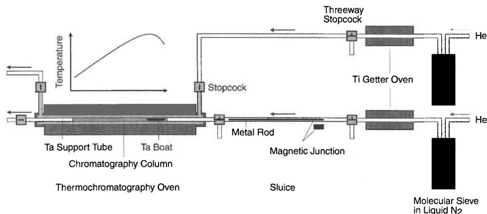
Fig. 1. The thermochromatographic apparatus.
