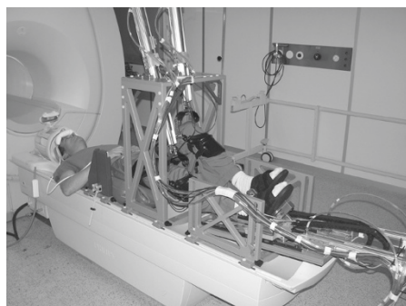
Figure 1 The fMRI compatible robotic stepping actuator MARCOS. Left: MARCOS in the 1.5T MR scanner. Right: Sketch of the MARCOS system (only 1 leg depicted for clarity). MARCOS is actuated by two pneumatic cylinders per leg. The reaction forces between the subject and the robot are measured through force sensors located in the knee orthosis attachment and the foot plate. The position of each cylinder piston is measured redundantly by optical encoders [26].
