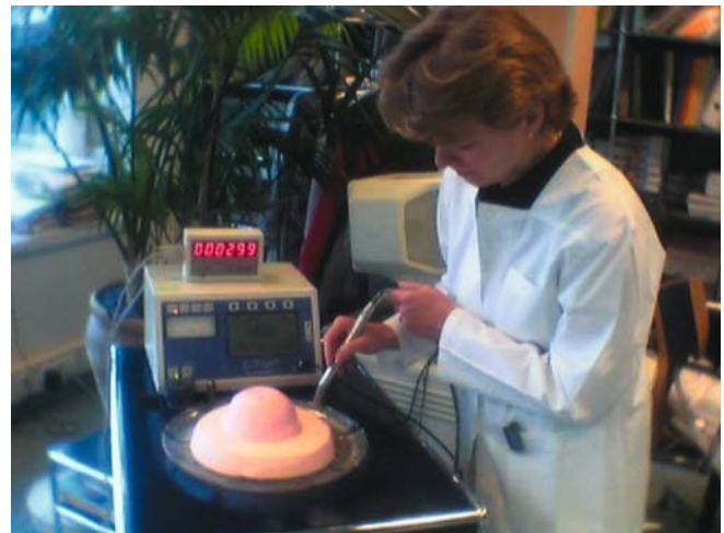
Fig. 1. Tracking the radioactive ‘sentinel node’ within the humanoid phantom with the gamma probe
