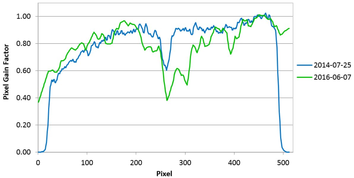
Fig. A.6. Pixel gain factors for each individual pixel on Row A for GS16. The 2014-07-25 and 2016-06-07 curves were measured early and late in the mission, respectively.
