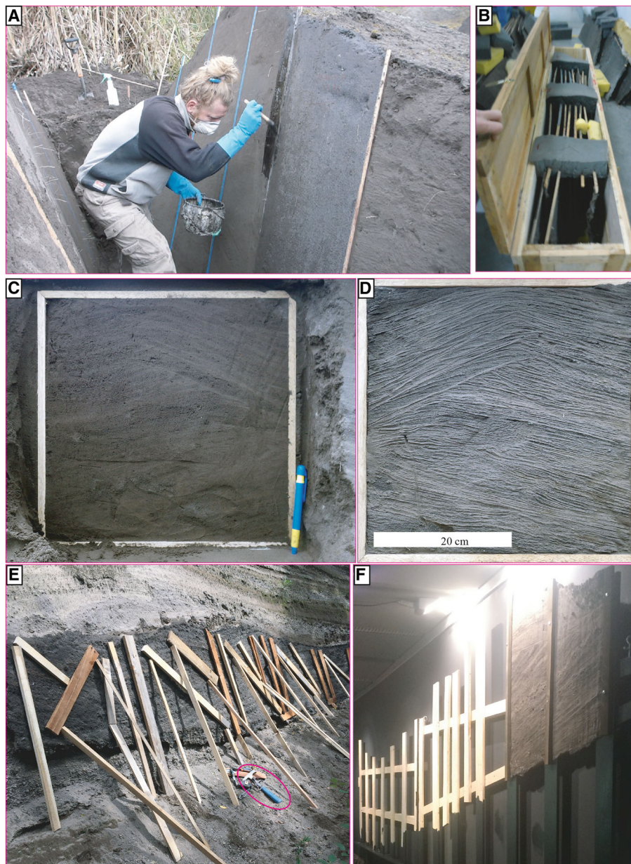
Fig. 1 a Impregnation of a bedform by simple brushing, Tungurahua 2006 deposits. Note delimitation of individual plates with wooden strips separated by sticky tape, flatness of the surface and slight angle to the vertical. b Sediment plates packed in boxes for shipping. c A natural outcrop and d the resulting sediment plate with enhanced detail level, Tungurahua 2006 pyroclastic currents, note that the exposed (inner side) of the plate is mirroring the outcrop view when taken out. For interpretation, see Douillet et al. (2015). e Lapilli-type sediment plate stabilized with mounting foam and wooden boards at Laacher See before cutting and extracting the plates from outcrop. f Wooden frames on which sediment plates were mounted during the exhibition "G'Schichten von Tungurahua"
