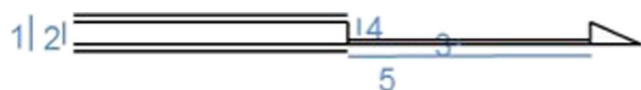
Fig. 1 Needle micro-mechanical characteristics. 1: needle external diameter, 4: needle tray height (comes from the extraction of 2–3) and 5: effective needle tray length
