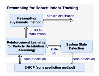
Figure 2: Reinforcement Learning Method for Robust Indoor Tracking Resampling.
