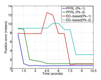
Figure 15: Scenario 1: Global Localization Failure recovery. Particles convergence time after localization failure
