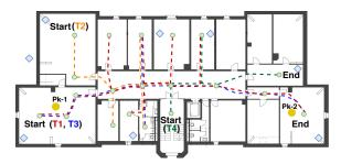
Figure 7: Trajectories definition in Scenario 1, circle yellow points are the kidnapped robot check points.
