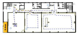
Figure 8: Trajectories definition in Scenario 2, yellow region is the area where particles are kidnapped.
