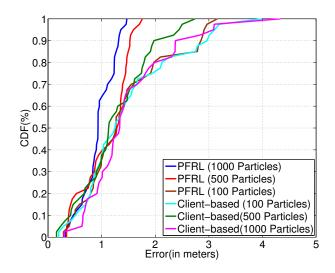
Figure 11: Impacts of particle numbers on performance of PFRL and client-based PFRL in scenario 1.
