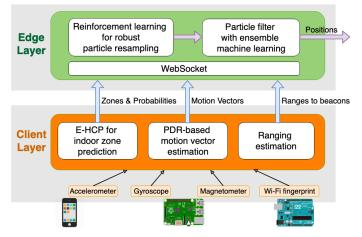
Figure 1: Distributed Machine Learning System Architecture for Reliable Wireless Indoor Positioning.
