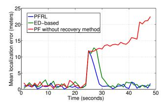
Figure 18: Scenario 2: Kinapping Robot Problem. Particles convergence time after a localization failure is detected.
