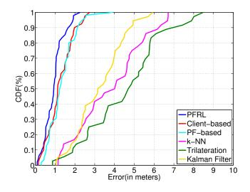
Figure 20: Scenario2: Localization error CDF of PFRL (1000 particles), Client-based (500 particles) NLS, k-NN and KF.
