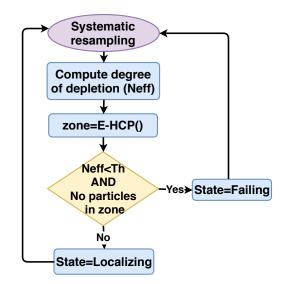
Figure 4: PFRL system state detection method flowchart.
