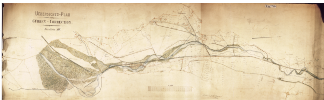
Plan of the natural course of the Gürbe River and the planned channel in Wattenwil, 1881.
