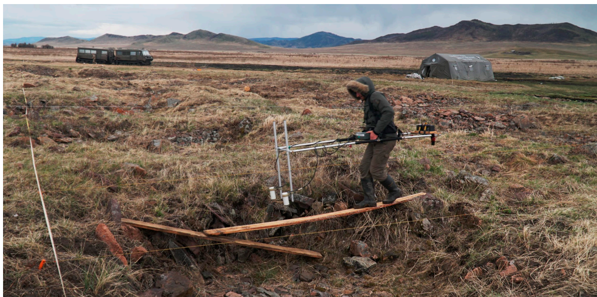
Figure 8. Wooden planks and a light weight geomagnetometry device made the survey on the burial mound possible. Ground-penetrating radar and geoelectric resistivity would not have been possible under these circumstances. Photo: T. Wallace.
