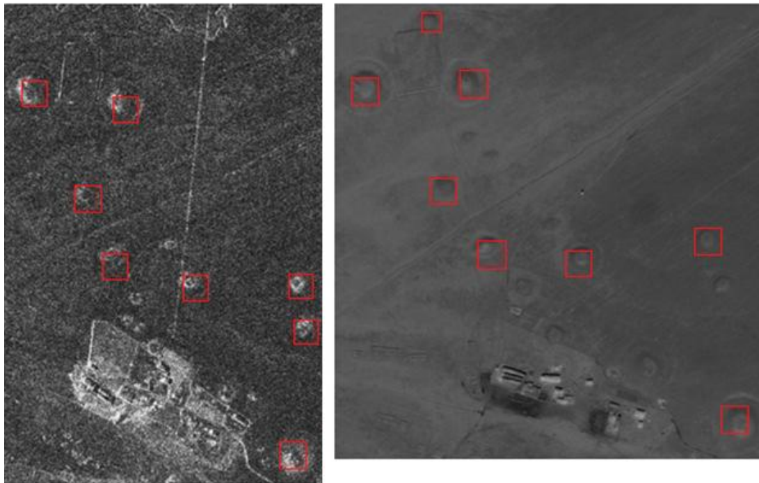
Figure 5. Example of classification results from TerraSAR-X staring spotlight data (left) and IKONOS-2 data (right)
