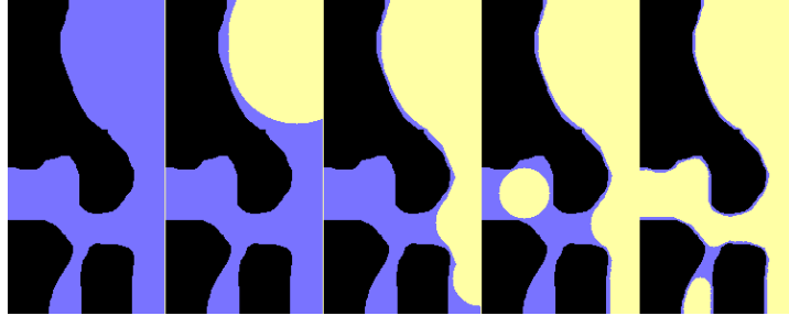
Figure 2: Illustration of a drainage process in a pore structure map. The sequence of frames from left to right corresponds to decreasing water potential. Drainage took place from all domain boundaries. The simulations included both, capillary effects (drainage of the core of pores with a decreasing radius) and surface adsorption effects (thinning of surface water films). Black: solid, blue: water, yellow: drained pore.
