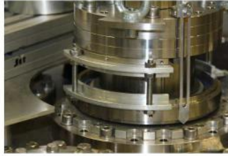
FIGURE 2.19: Photo of the new height adjustable spacer which allows for a precise z setting of the sample chamber.
