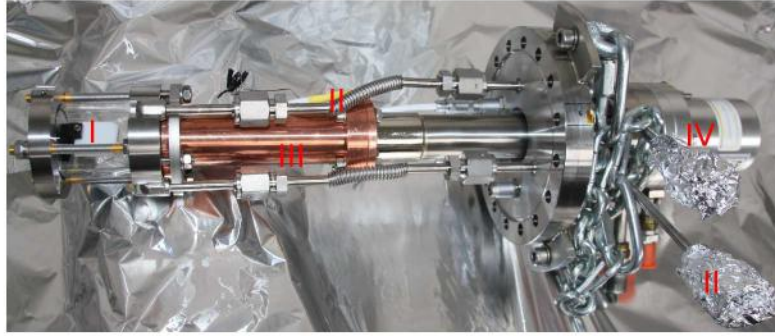
FIGURE 2.6: Photo of inner vessel with the quartz glass tube (I), the Xenon supply lines (II), the copper part which is used for the Xenon liquefaction (III) and the PTR itself (IV). Furthermore visible are the chains that are used to lift the tube with the pulley system, a PTFE sample in the sample holder and the top flange of the inner vessel.
