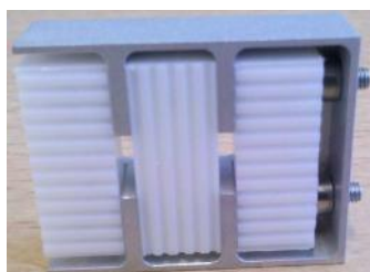
FIGURE 2.32: Photo of the grooved XENON1T reflector sub samples mounted in the sample holder. The samples will be measured in one measurement run. The right, thus lowest sample was replaced later with the reference sample B.
