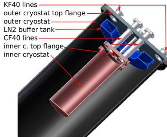
FIGURE 3.1: CAD image with an overview over the main components of the Bern LXe test platform. The outer cryostat is shown in black, the inner cryostat in brown and the LN2 tank in blue. The top flange of the outer cryostat with 2 of the 5 KF-40 flanges is shown in grey and the top flange of the inner cryostat is shown in brown with 2 of 3 CF-40 and the one CF-16 flange going through the top flange.
