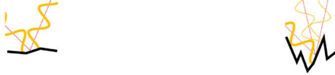
(A) Micro-surface which yield to a flat surface and high reflectance. (B) Micro-surface which are strongly tilted to the surface and low reflectance.
