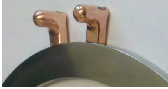
FIGURE 3.23: High voltage connectors (copper parts), specially developed for the anode HV supply. The field shaping ring is about 3 mm thick.
