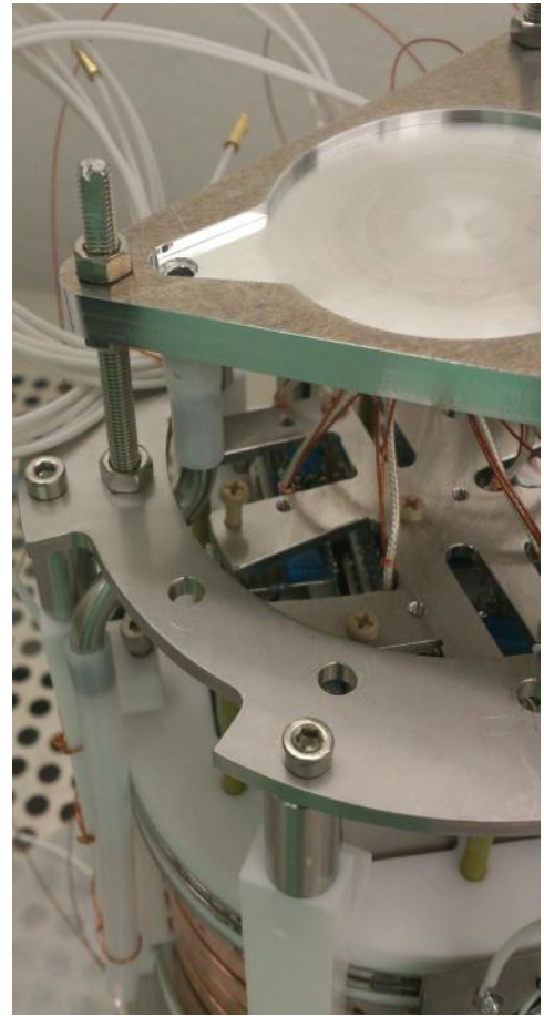
(B) Funnel above the TPC, which collects the LXe and the PTFE pipe that guides the LXe to the bottom of the inner cryostat.
