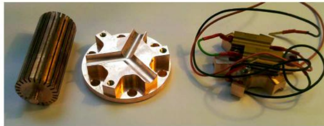
FIGURE 3.5: Photo of the cold finger, which sits in the inner cryostat. Left to right: slitted cold finger, cold finger top flange, top cap of the flange.
