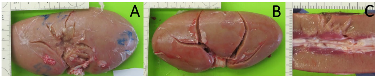
Fig. 2 Typical damage of the kidney corresponding to AIS 3: (A) impact side of the kidney, (B) opposite side of the impact, (C) cut through the kidney showing the damaged tissue with intact medulla and collecting system. Impact energy = 32 J, gelation layer thickness = 2 cm
