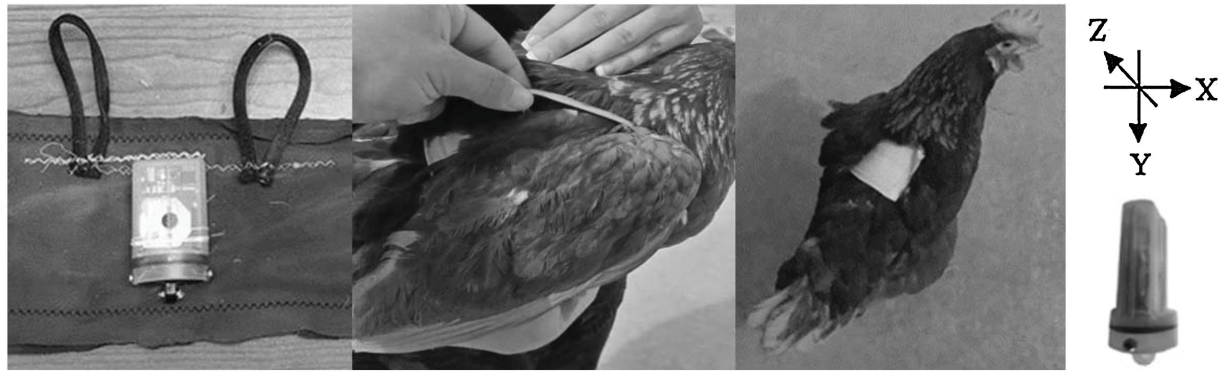
Figure 2. A fabric vest was used to secure the accelerometer to the hen. Vests were wrapped around hens' bodies behind the wings and secured using Velcro. Elastic bands around the base of the wings ensured the vest did not rotate or slip off the hen. The accelerometer was oriented so the X axis captured a hen's forward and backward movement and the Z axis captured vertical movement.
