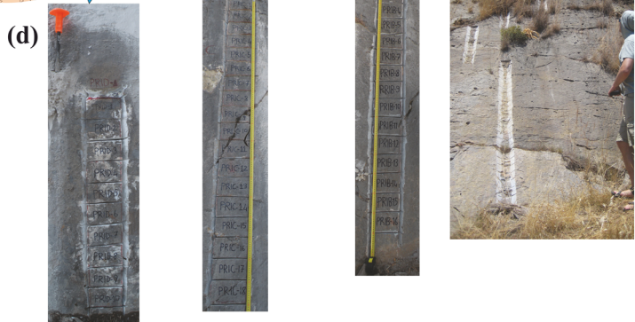
Figure 7. (a) Field view of the Priene–Sazlı Fault scarp at the base of the escarpment. (b) More detailed view of fault scarp with positions of continuous sampled strips A, B, C and D. The sampled surface is the lowest exposed surface of the successive scarp system. (c) Schematic sketch of fault scarp surface representing four sampled strips. (d) Fault scarp surface showing sampling slabs along strips A, B, C, and D. (e) Schematic sketch showing important parameters of the fault scarp for modeling, including scarp height, scarp dip, colluvium dip, top surface dip, and density of the bedrock and colluvium. Red dashed line shows the sampled surface.
