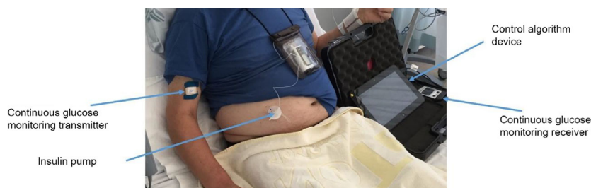
FIGURE 1 Automated fully closed-loop insulin delivery prototype (FlorenceD2W-T2) used by the woman in our case report (photo obtained with consent)
