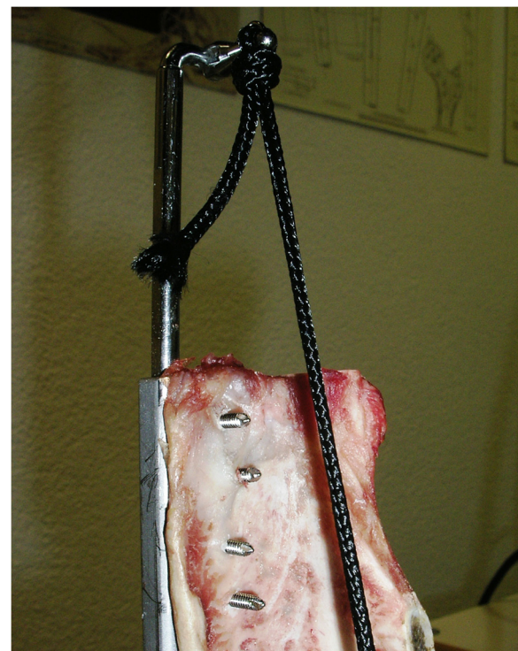
Figure 4 The setup of the loading direction made up in line with the sheep's infraspinatus muscle.
