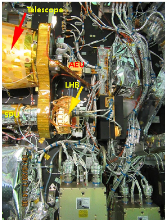
Fig. 5 BELA instrument on the spacecraft. The baffles can be seen on the left (upper) part of the image. The yellow side of the aluminium honeycomb baseplate is also evident. The laser head box is just to the right of the baseplate
