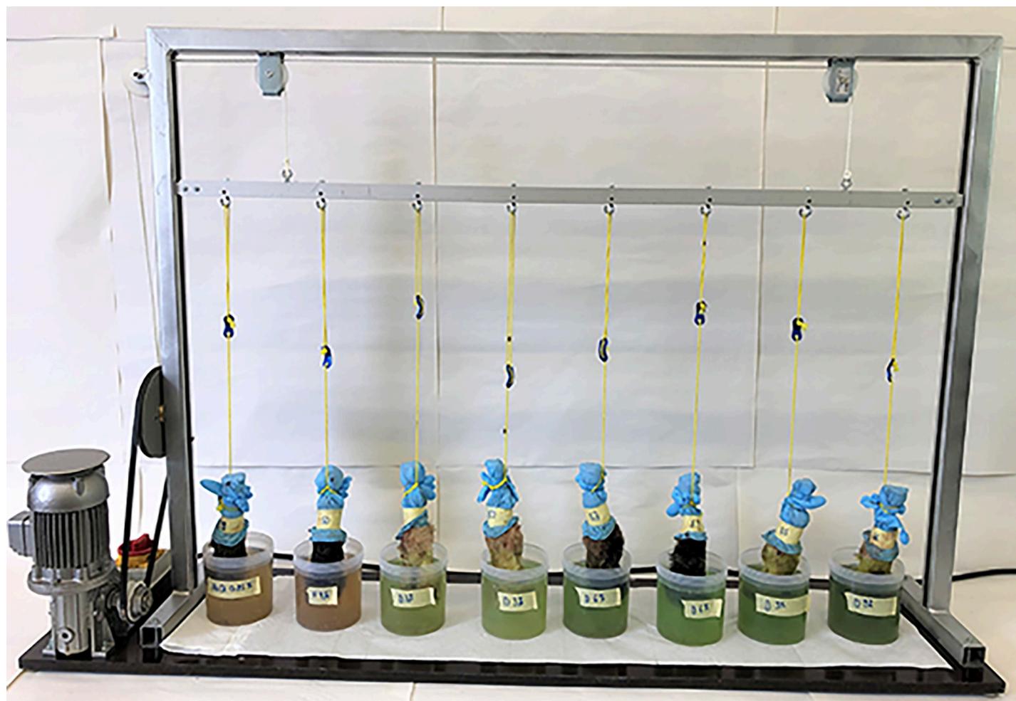
Fig 1. Foot-dipping machine. The foot-dipping machine simulates the movement of alive sheep feet in disinfectant footbath solution.
