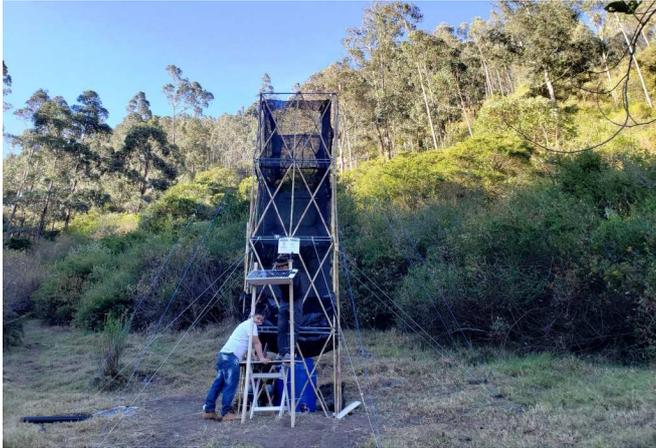
Fig. 9 Installation of sensors fog collector system
