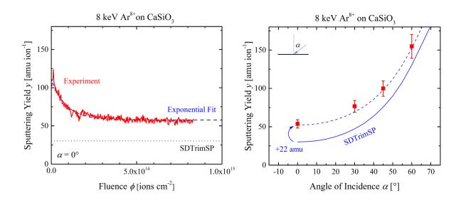
Figure 6: Left: Fluence dependence of the sputtering yield under continuous  $Ar^{8+}$  irradiation, which can again fitted with an exponential decrease. Fluences up to about  $8\times10^{12}$  ions cm<sup>-2</sup> are affected by thermal stabilization
