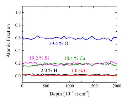
Figure 2: ToF-ERDA analysis of a 700 nm  $CaSiO_3$  film for the first  $2000 \times 10^{15}$  at cm<sup>-2</sup> (roughly 260 nm), where this method can reliably probe the elemental composition of the sample. The analysis shows that the concentrations of Ca (green), Si (pink) and O (blue) are close to  $CaSiO_3$ . Only minor contaminations of H (black) and C (red) are observed.
