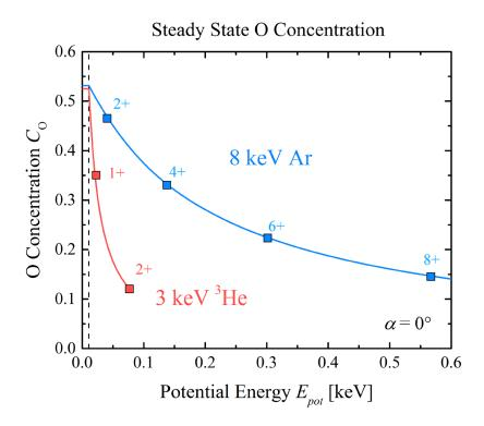
Figure 9: Calculated steady state O concentrations for normal incidence irradiation are plotted over the ion's potential energy. For Ar (blue), O depletion is not as severe as for He (red) because more Ca and Si is removed by kinetic sputtering. For He (red), potential sputtering is dominant already at lower potential energy and O depletion is much more significant.
