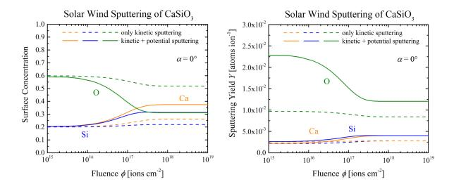
Figure 10: Left: Fluence dependence of the calculated surface concentration changes resulting from solar wind sputtering of CaSiO<sub>3</sub>, assuming a solar wind
