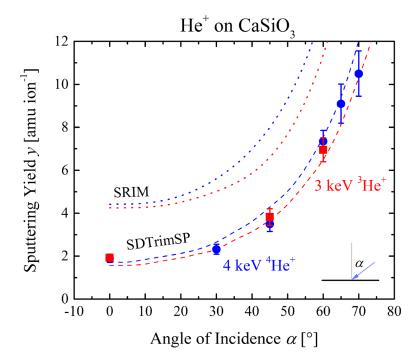
Figure 4: Comparison of the sputtering yields for 3 keV  $^3\mathrm{He^+}$  (red) and 4 keV  $^4\mathrm{He^+}$  (blue) bombardment. Experimental results are plotted for different angles of incidence together with simulation results from SDTrimSP (dashed lines) and SRIM (dotted lines).
