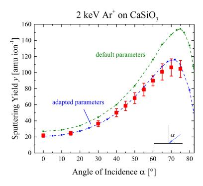
Figure 3: Comparison of different SDTrimSP simulations with experimental results (red) for 2 keV Ar+ sputtering yields. Default parameters (green) overestimate the measured yields, while the adapted parameters (blue) give a better agreement.
