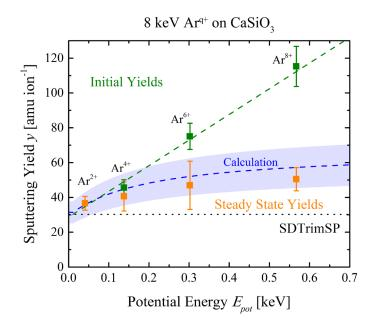
Figure 7: Ar sputtering yields for different potential energies of the ions, measured for the charge states 2+, 4+, 6+ and 8+. Sputtering yields at the beginning of the irradiation show a linear dependence (green) with  $E_{pot}$ . Steady state sputter yields depend much less on  $E_{pot}$  (orange). The calculation for dynamic potential sputtering is able to reproduce the measured steady state yields very well (blue dashed line, shaded area represents an uncertainty estimate, see Section 4).
