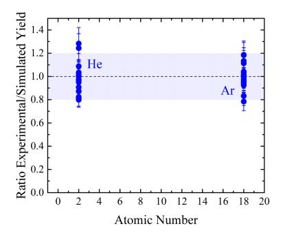
Figure 11: Compilation of the ratio between experimental and simulated sputtering yields using the  $CaSiO_3$  bulk density and an adapted surface binding energy. Measured data includes different kinetic energy for  $^3He$  (3 keV),  $^4He$  (1 keV, 2 keV, 4, keV) and Ar (1 keV, 2 keV, 4 keV). Most ratios lie within the blue shaded area of 0.8 - 1.2.
