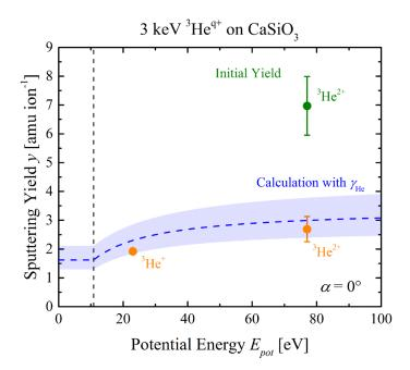
**Figure 8:** Comparison of the sputtering yields for  ${}^{3}\text{He}$  sputtering plotted over the ion's potential energy. Measured steady state yields (orange) are compared to calculation results (blue dashed line) using the initial  ${}^{3}\text{He}^{2+}$  yield (green).
