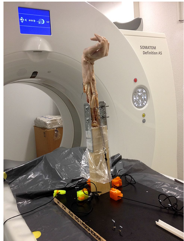
Fig. 2 Mounting of the cadaver arm with loaded tendons with tension springs (50 N)
