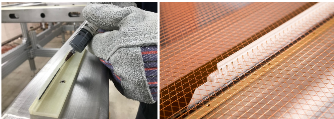
Figure 18. Left: the adjustable base slats of the combs being epoxied in place after their level has been set. Right: a finished stack of combs encapsulating the wires.
