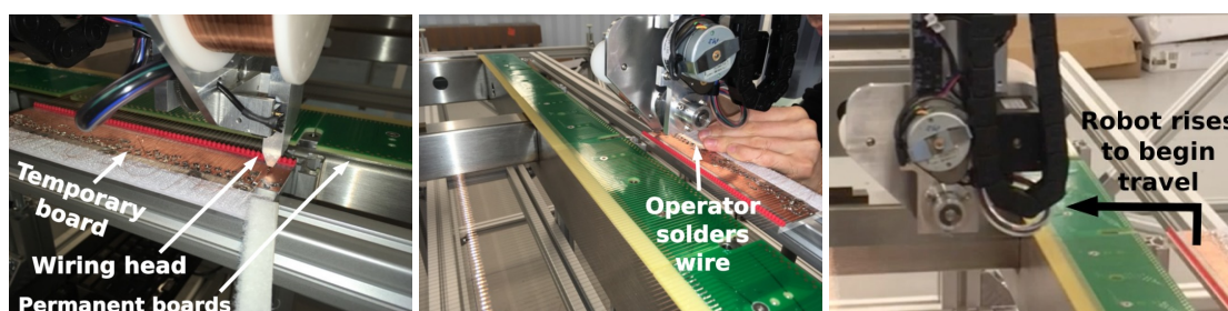
Figure 26. Steps 1–3 of the wiring process. The wiring head is positioned and one end of the wire is soldered in place.
