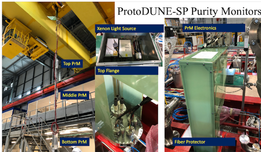
Figure 8.17. The ProtoDUNE-SP purity monitoring system.
