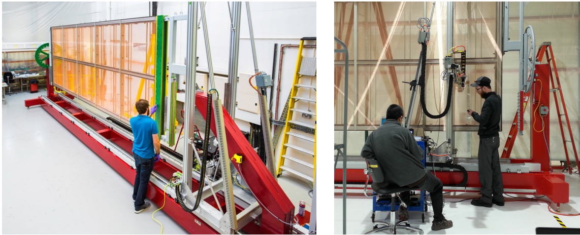
Figure 2.33. Left: partly wired ProtoDUNE-SP APA on the winding machine at Daresbury Lab, UK. Right: partly wired ProtoDUNE-SP APA on the winding machine during wire tension measurements at PSL.
