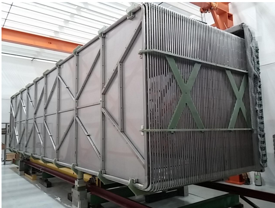
Figure 4. Exterior view of the MicroBooNE time projection chamber showing the cathode frame, structural supports, and the field-cage, before it was placed in the cryostat. There are 63 field-cage rings supported by horizontal G10 beams. Taken from ref. [2].
