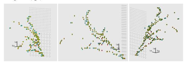
**Figure 2.** A cosmic ray-induced shower recorded with the LBNL LArPix equipped charge-readout system shown in Figure 1 in the Bern pixel demonstration LArTPC. The same 3D event is shown from three different angles.
