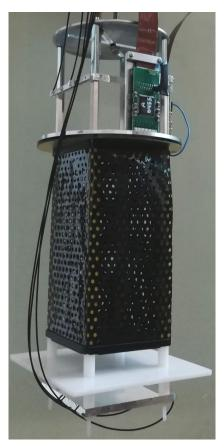
Figure 3. The Bern field-shell demonstrator LArTPC. The field-shell and cathode are made from  $\sim$ 50 µm resistive kapton foil. For this test, the field-shell was perforated to allow the purification of the LAr within the active volume. The Time Projection Chamber (TPC) has a 7 cm  $\times$  7 cm footprint and a 15 cm drift length. A bias of up to -23 kV was applied to the cathode to generate a 1.5 kV cm $^{-1}$  drift field [34].
