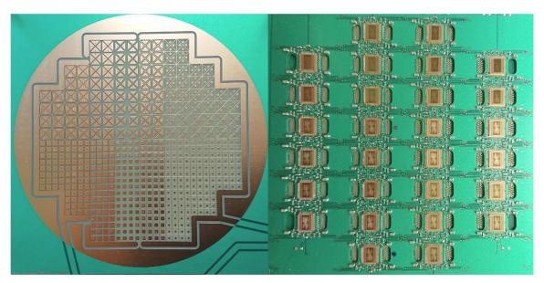
**Figure 1.** A prototype pixelated charge-readout Printed Circuit Board (PCB) developed as part of the ArgonCube R&D programme. The PCB has 832 pixels with various pad geometries, to identify optimal dimensions (**left**). Lawrence Berkeley National Laboratory's (LBNL) LArPix Application-Specific Integrated Circuits (ASICs) are mounted directly on the rear of the PCB, providing cold signal digitization (**right**).
