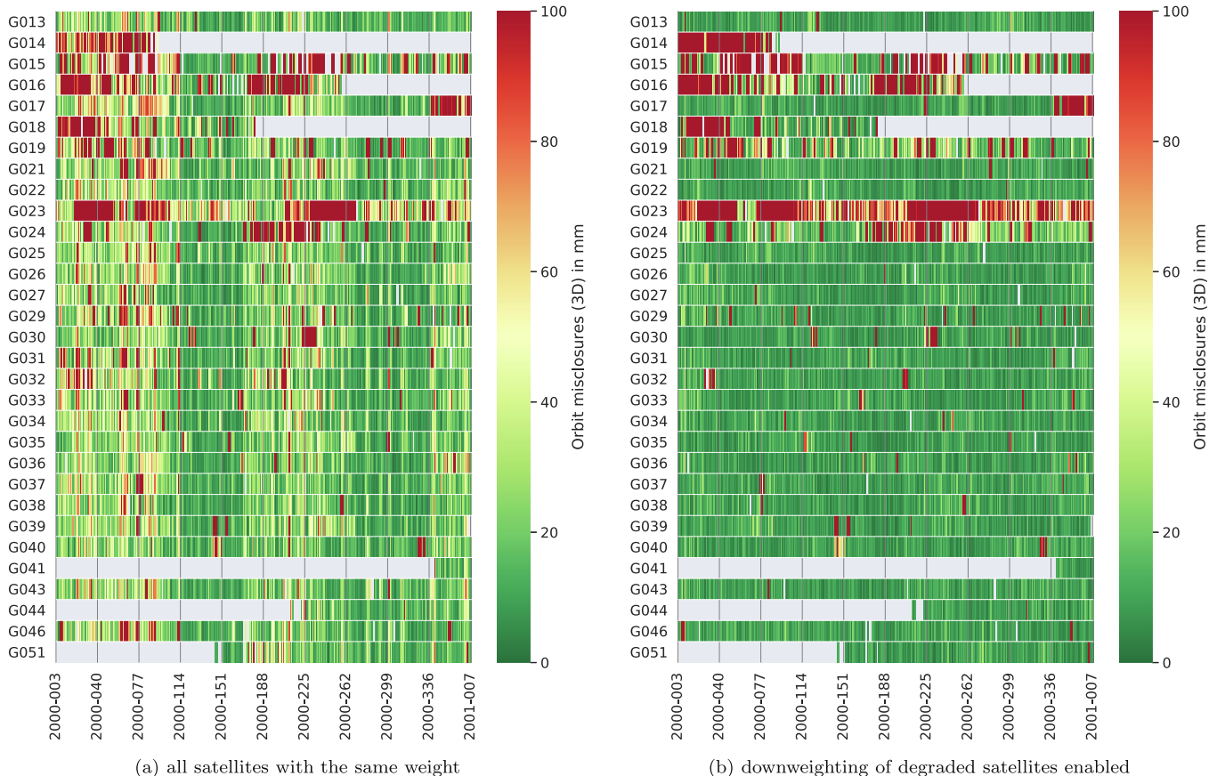
Fig. 10. Orbit misclosures from three-day solutions during the year 2000; the satellites are sorted according to their SVN.
