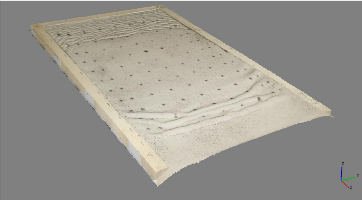
Figure 3: Example of model 3D rendering obtained after SfM mesh interpolation (Model H, t=48h). Note that these files are for 3D visualization, but do not allow for analysis (see Fig. 4).
