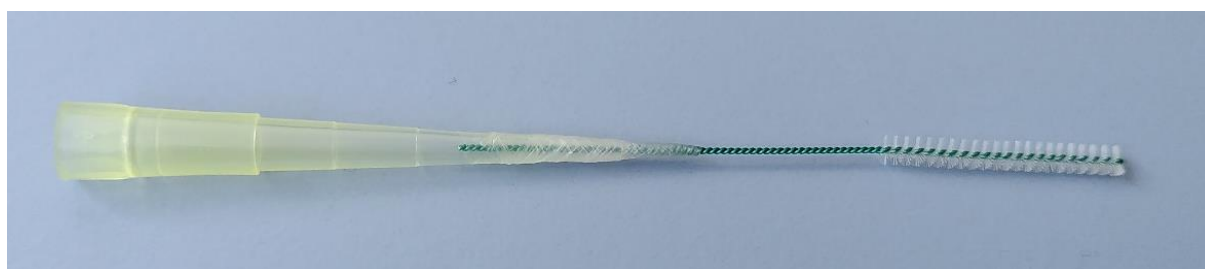
Figure A1. Interdental brush elongated by attaching a 200- \mu L pipette tip with parafilm.
