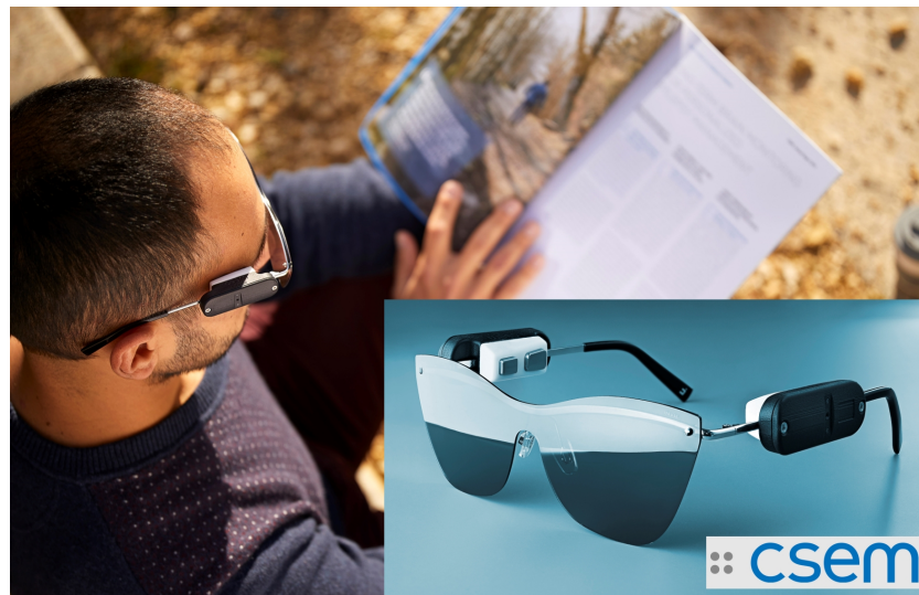
Figure 4. The ULTEEM recording system developed by CSEM (Swiss center for electronics and microtechnology) is integrated into glasses and thus minimizes obtrusiveness and stigmatization.
