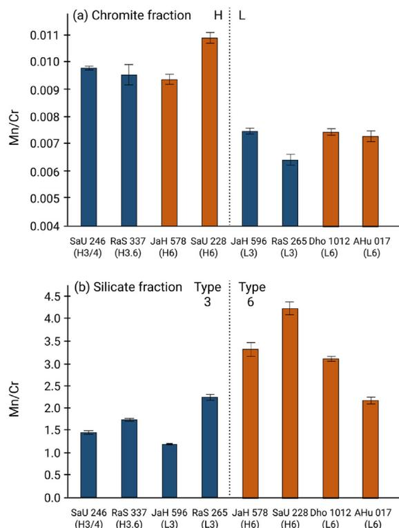
Fig. 3. (a) Mn/Cr ratios in chromite fractions. The ratios are systematically higher in H chondrites than L chondrites (b) Mn/Cr ratios in silicate fractions. The dashed line highlights the dichotomy between lower Mn/Cr ratios in type 3 samples and higher Mn/Cr ratios in type 6 samples. Uncertainties associated with the Mn/Cr ratios determined by replicate measurements are shown as 2SE.
