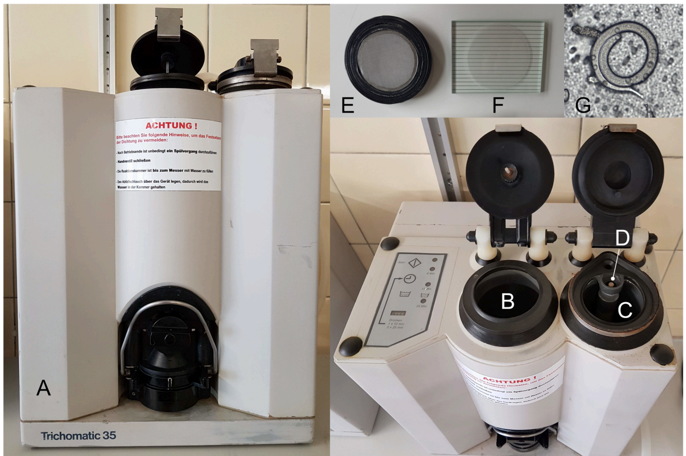
Fig. 1. A: Trichomatic instrument (Foss GmbH, Germany); B: reaction chamber; C: water chamber; D: HCl chamber; E: sieve; F: polycarbonate filter on glass for microscopic observation; G: polycarbonate filter with Trichinella larva.
