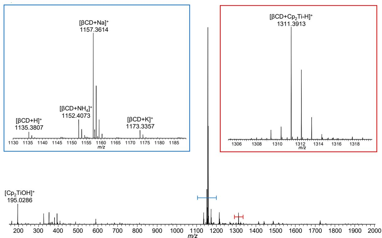
**Figure 4.** Full scan mass spectrum of the mixture of  $\beta$ -cyclodextrin and titanocene dichloride showing the peak indicating an interaction between the two compounds (red inset), as well as the hydrolyzed titanocene, and cationized  $\beta$ -cyclodextrin (blue).
