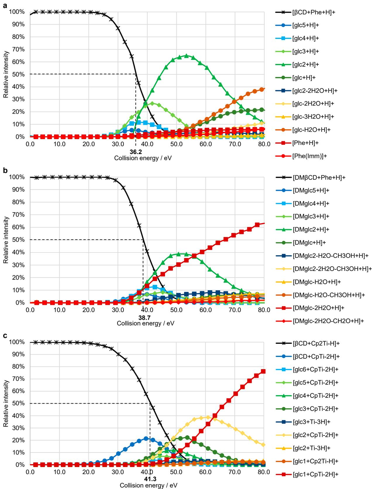
**Figure 7.** Breakdown curves recorded for HCD experiments of: (a)  $[\beta\text{CD} + \text{Phe} + \text{H}]^+$  ( $m/z$  1300.48), (b)  $[\text{DM}\beta\text{CD} + \text{Phe} + \text{H}]^+$  ( $m/z$  1496.70), (c)  $[\beta\text{CD} + \text{Cp}_2\text{Ti-H}]^+$  ( $m/z$  1311.40). Fragment ions with a maximum relative intensity < 2% are not displayed. The dashed lines indicate the  $\text{CE}_{50}$  values.
