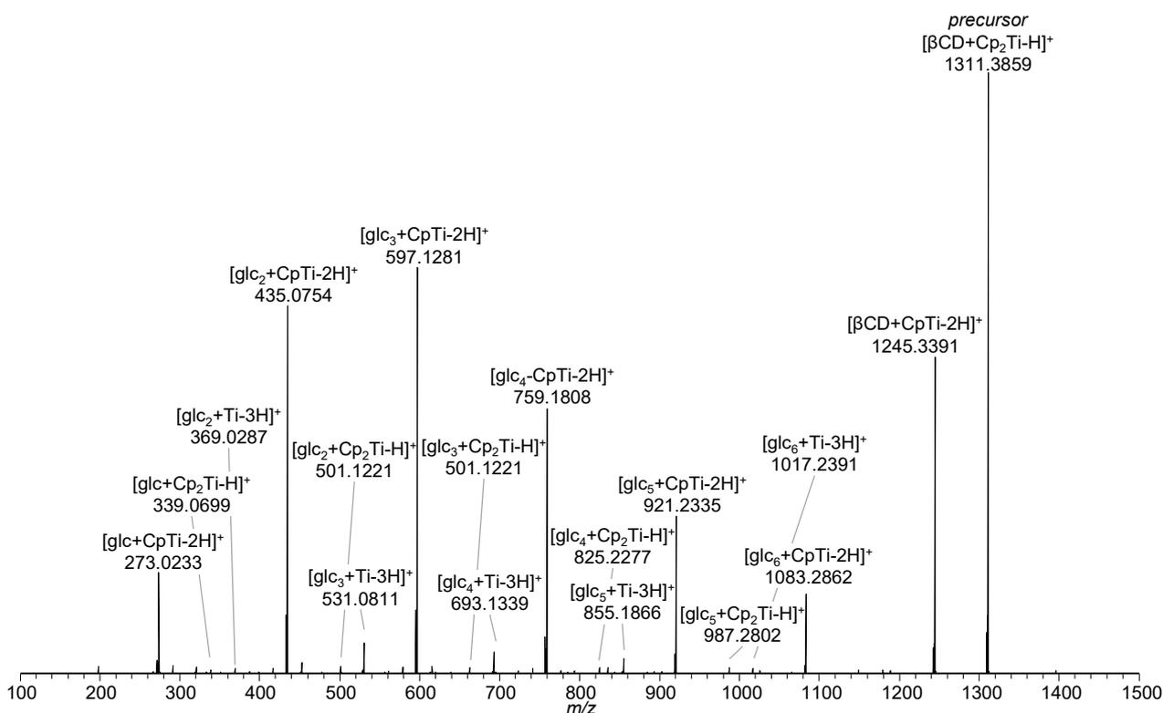
**Figure 5.** HCD mass spectrum of  $[\beta\text{CD} + \text{Cp}_2\text{Ti-H}]^+$  ( $m/z$  1311.40) at 47 eV (20% NCE) showing the loss of one or two cyclopentadiene moieties ( $\text{C}_5\text{H}_6$ ) and the decomposition of  $\beta$ -cyclodextrin into its subunits, still interacting with titanocene species.
