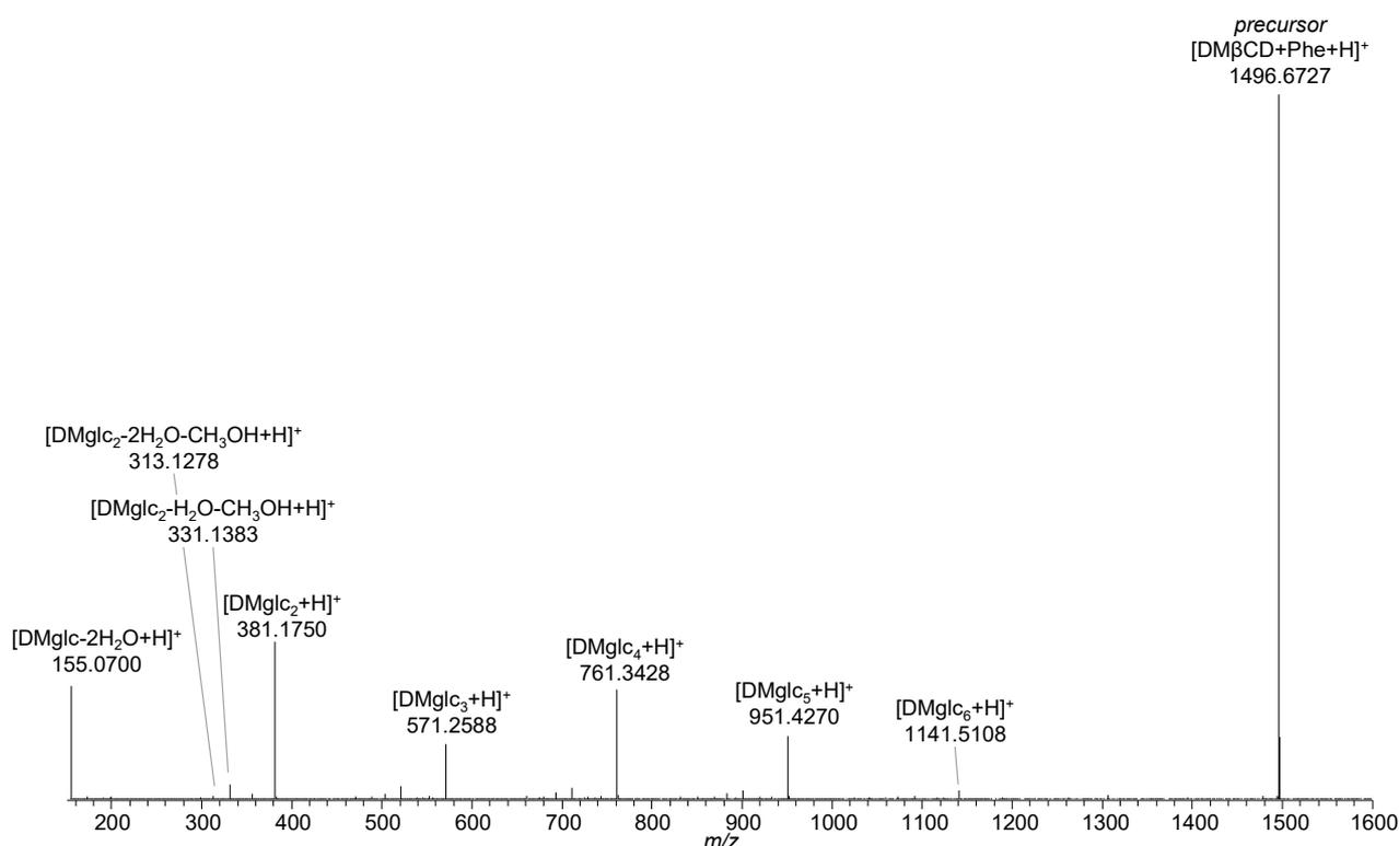
**Figure 6.** HCD mass spectrum of [DM $\beta$ CD + Phe + H]<sup>+</sup> ( $m/z$  1496.70) at 40 eV (15% NCE) showing the separation of the precursor ion and subsequent decomposition of DM $\beta$ -cyclodextrin into its subunits [DMglc<sub>n</sub> + H]<sup>+</sup>.
