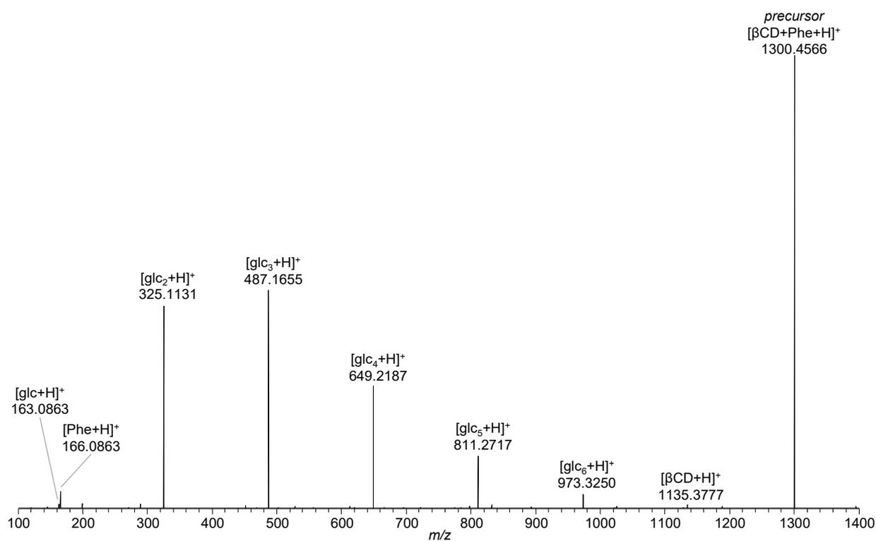
**Figure 3.** Higher energy collision induced dissociation (HCD) spectrum of  $[\beta\text{CD} + \text{Phe} + \text{H}]^+$  ( $m/z$  1300.48) at 37 eV (16% normalized collision energy (NCE)) showing the separation of the precursor ion into  $[\text{Phe} + \text{H}]^+$ ,  $[\beta\text{CD} + \text{H}]^+$ , and  $\beta$ -cyclodextrin fragment ions  $[\text{glc}_n + \text{H}]^+$  ( $n = 1-6$ ).
