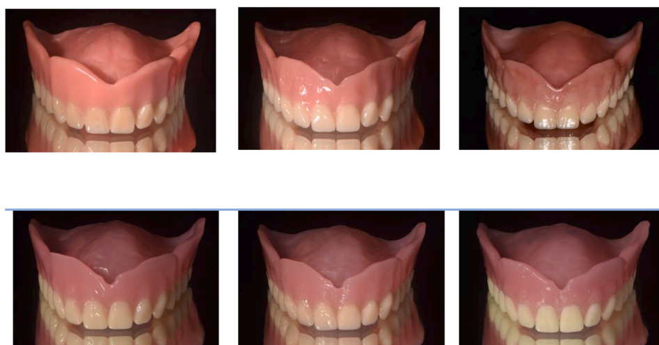
Fig. 2. A-F (from right to left). Examples of the specimens produced by the six different manufacturing methods: Conventional: A. Flask-pack-press (FP), B. Injection Molded (IM), C. Customized finish (NG) and CAD-CAM: D. Milled base with prefabricated, bonded teeth (M), E. fully milled (FM), F. Rapid-prototyped (P).
