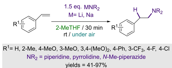
Scheme 13. Hydroamination of vinylarenes with alkali-metal amides under air and at room temperature, using 2-MeTHF. [15b]
