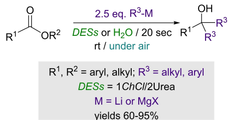
Scheme 6. Chemoselective addition of polar organometallic reagents (RLi/RMgX) to esters under air, at room temperature and using either water or ChCl -based eutectic mixtures as reaction media for the synthesis of symmetric tertiary alcohols. [11]
