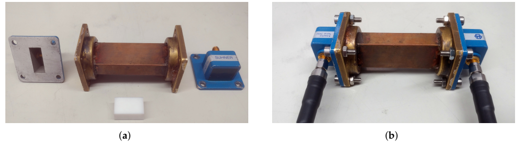
Figure 3. Waveguide as sample holder, MUT, and connection with the network analyser. (a) WR90 waveguide with coaxial adaptors and PTFE material sample; (b) assembled waveguide connected to the network analyser.
