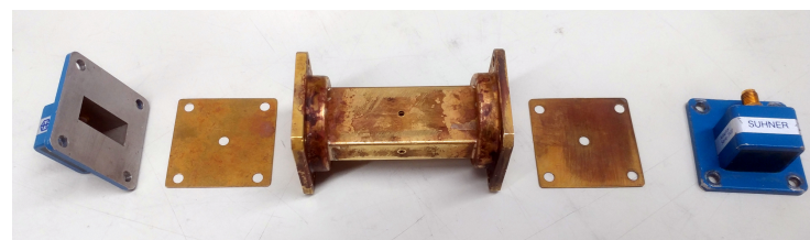
Figure 4. WR90 waveguide with coupling irises and coaxial to waveguide adaptors. The small holes in the waveguide’s broad and narrow walls are used for sample insertion.
