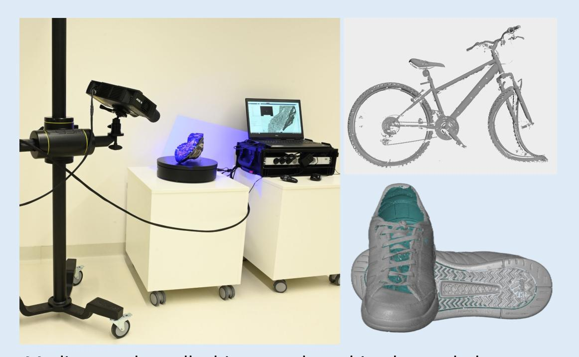
Medium and small objects such as bicycles and shoes are documented by means of **structured-light scanning** using various systems adapted to the object size and required level of detail. Standard 2D photo documentation is still a matter of course.
