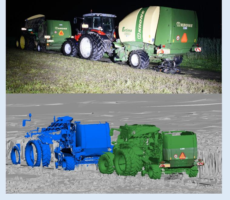
The accident site and large objects such as agricultural vehicles are documented using laser scanning and photogrammetry.
